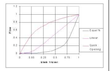
The graph below provides three typical inherent flow characteristics of control valves described in
