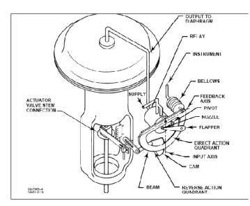
Large no of design variations are available for each of the above functions. Incorporations of other 'addons' like variation in gain (amount of air into the actuator that will be e d m 0 v compared to signal pressure), split operation, zero adjustments (to take care of slackness). travel adjustment( for various valves) etc. also introduce design
